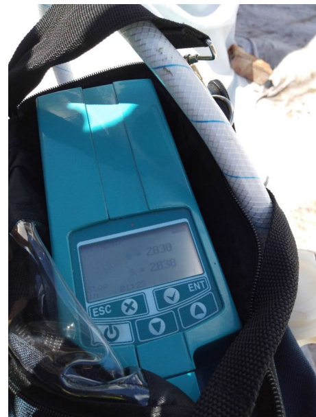
Fig. 1 LUMEX RA-915 mercury analyser
