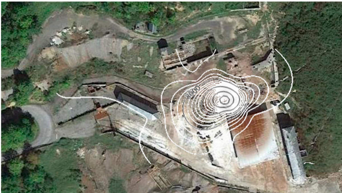
Figure 5. Survey 2's gaseous mercury concentration, (white lines are concentration isolines around the focus).
