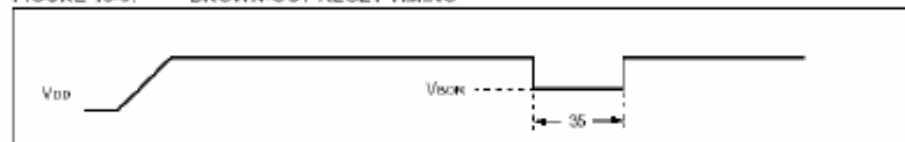
FIGURE 15-9: BROWN-OUT RESET TIMING
