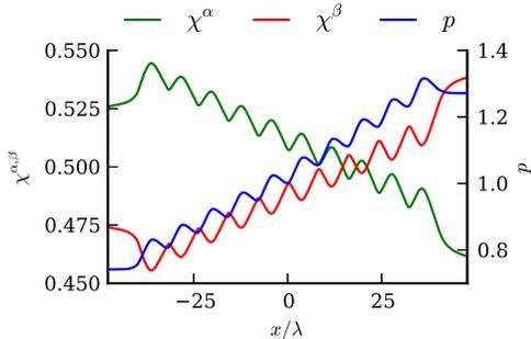
Figure 12: Pressure and relative concentrations along the multistage pump axis.
