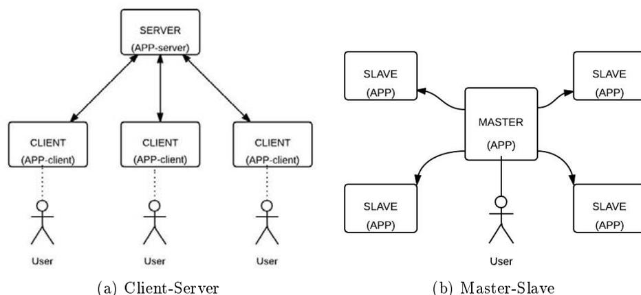
Figure 1: Cluster display wall architectures
