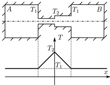
Figure 7: Scheme of the Knudsen pump.
