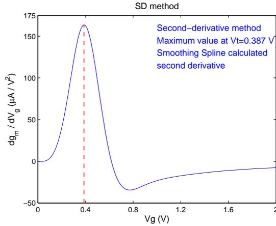
Figure 1: TCM or SDM using  $I_d - V_g$  characteristics. In this method we seek the maximum of the second derivative of the  $I_d - V_g$  curve. This value is taken as the threshold voltage of the device.
