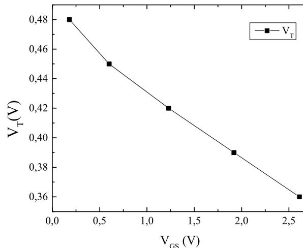
Figure 6: Calculated threshold voltage  $V_T(V)$  versus gate voltage,  $V_{GS}(V)$ , obtained by means of the transconductance change method, using the WENO approximations of the derivatives and a linear interpolation at specific points.
