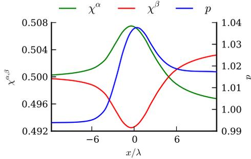
Figure 9: Pressure and relative concentrations along the pump axis.
