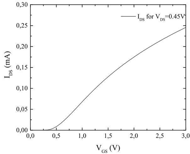
Figure 3: Drain current  $I_d(A)$  versus gate voltage,  $V_g(V)$ , for a constant drain voltage  $V_d$ .
