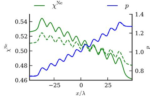
Figure 13: Pressure and relative concentration of light gas along the pump axis.
