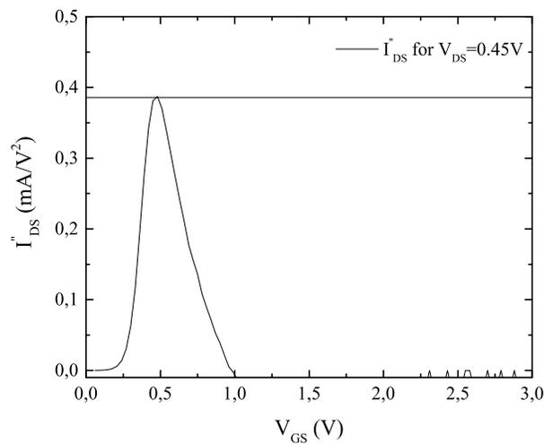
Figure 5: Approximation of the maximum of the second derivative  $I''_d(A/V^2)$  versus gate voltage,  $V_g(V)$ .
