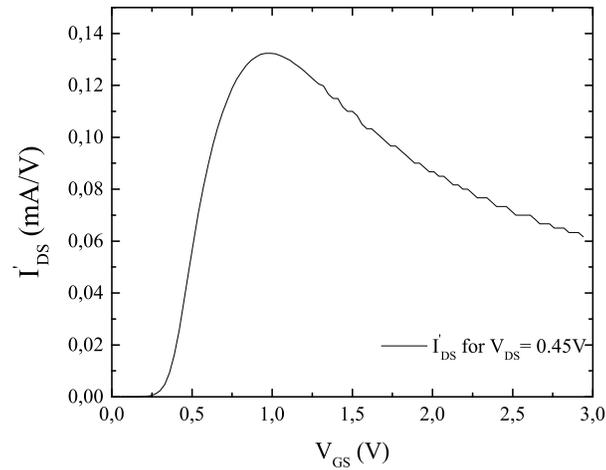
Figure 4: Approximation of the first derivative  $I'_d(A/V)$  versus gate voltage,  $V_g(V)$ , using the WENO procedure.
