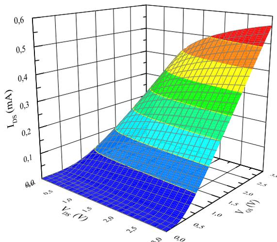
Figure 2: Drain current versus gate voltage and drain voltage for the transistor simulated.
