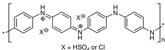
Fig. (2). Structure of the conducting polyaniline polymer.
