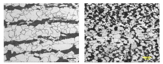
Figure 9: Microstructure of steel in its Hot Rolled Raw State Condition (a) and the steel tested at 800°C and 5.5x10<sup>-5</sup> s<sup>-1</sup> strain rate (b)
