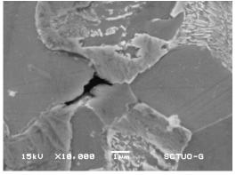
Figure 11: Decohesions or microcavitations between the ferrite and pearlite during superplastic deformation (R-shaped crack) (a) and as a consequence of a conventional high-temperature deformation (decohesions between matrix and hard constituent) (b).
