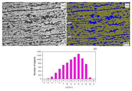
Figure 6: Hot rolled raw state microstructure (a), detected ferrite phase (b) and ASTM G ferrite grain size distribution histogram (c)
