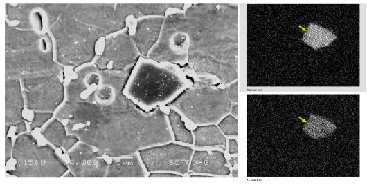
Figure 12: SEM micrograph showing a titanium carbonitride and niobium carbide.
