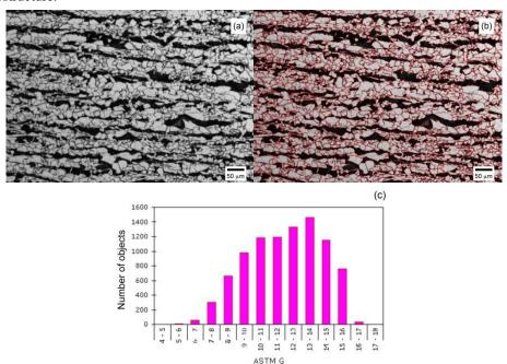
Figure 5: Hot rolled raw state microstructure (a), detected grain pattern (b) and ASTM G grain size distribution histogram (c)
