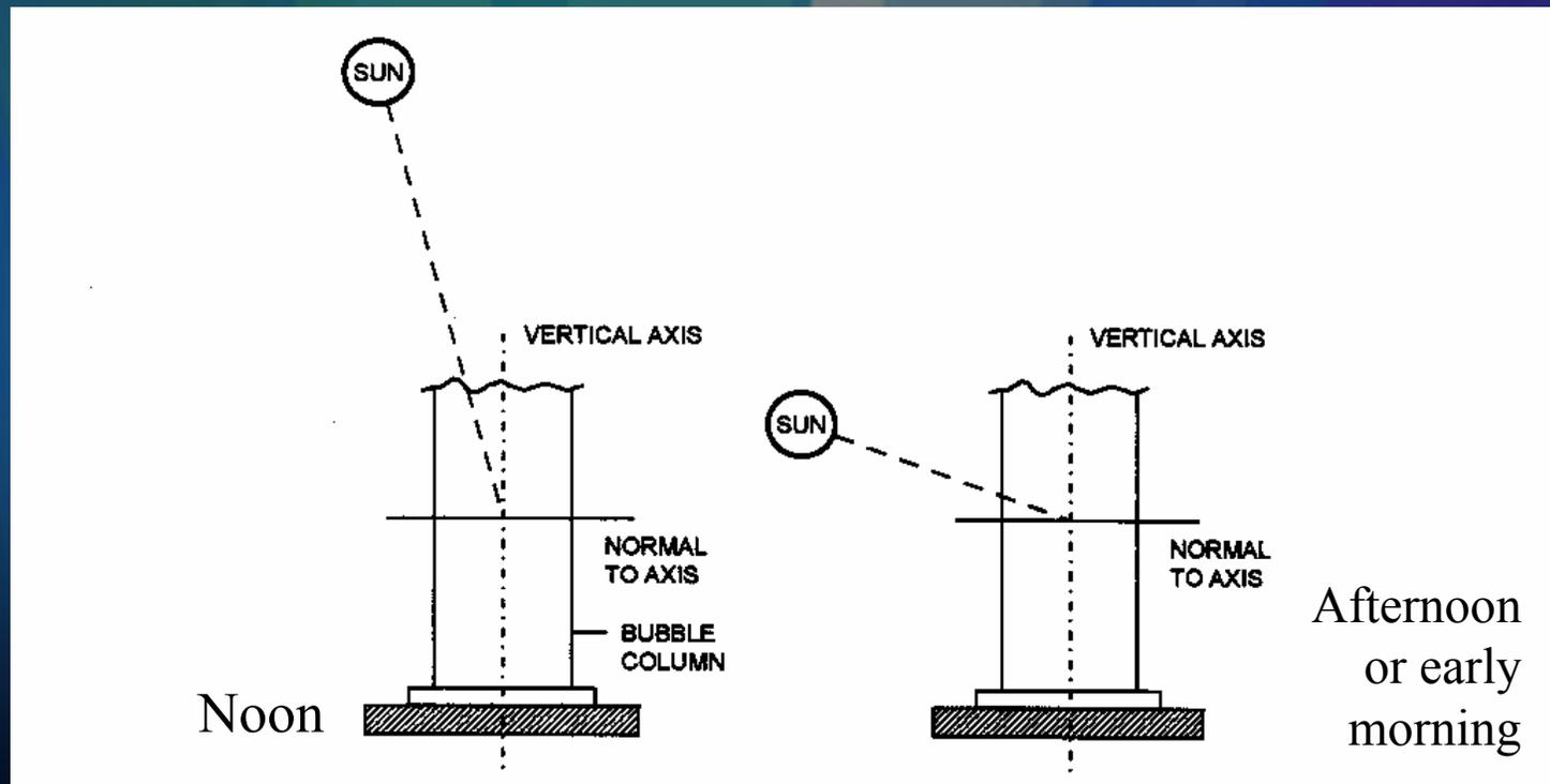
The amount of solar energy absorbed is lower than for horizontally placed reactor
