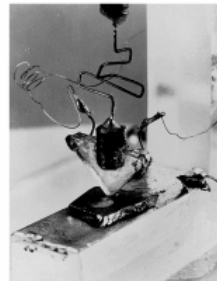
First Transistor, Bell Lab, 1947
