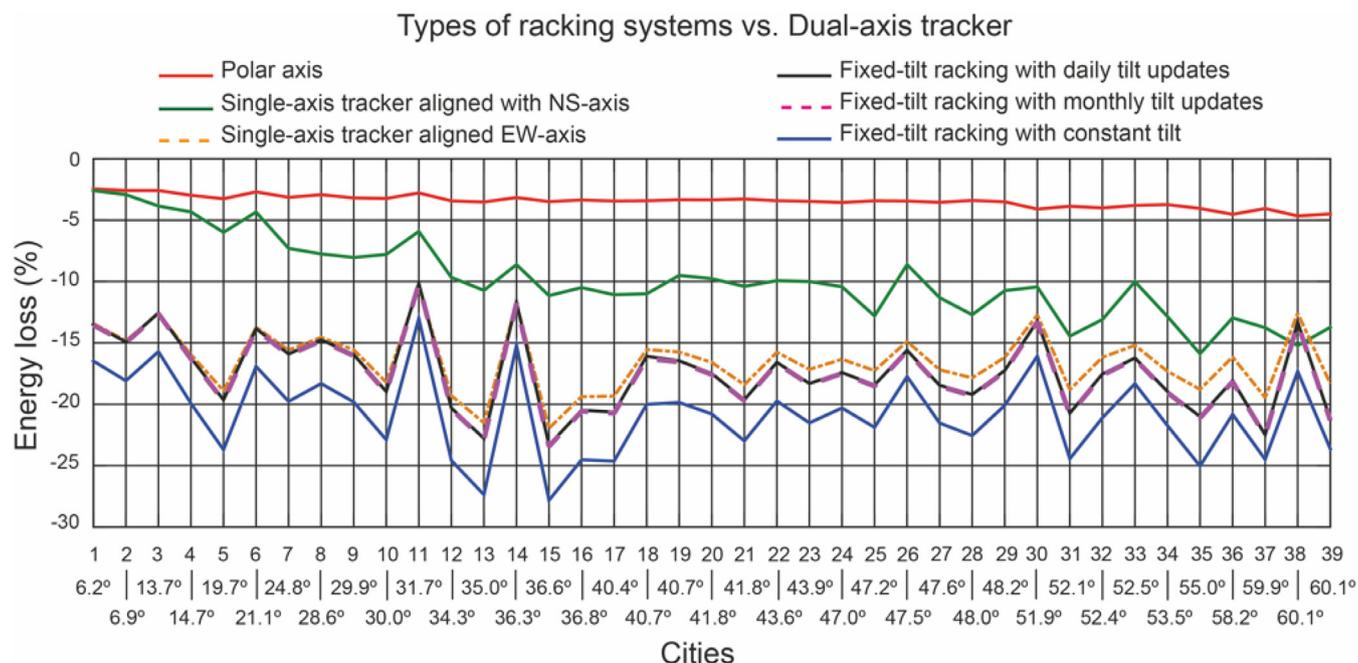
Fig. 10. Ratio of energy loss with respect to the dual-axis tracker. Notice that the daily and monthly plots overlap.
