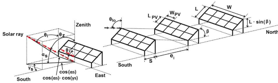
Fig. 3. Longitudinal and transversal study of the installation.
