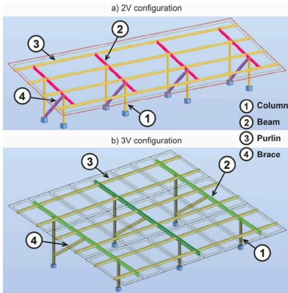
Fig. 1. Solar array mounting frame structural arrangement types.
