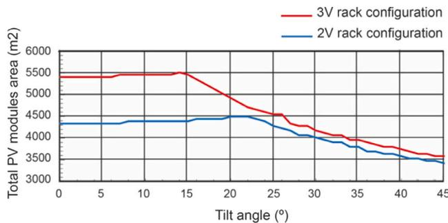
Fig. 8. Total PV modules area,  $A_{TPV}(\beta)$ .
