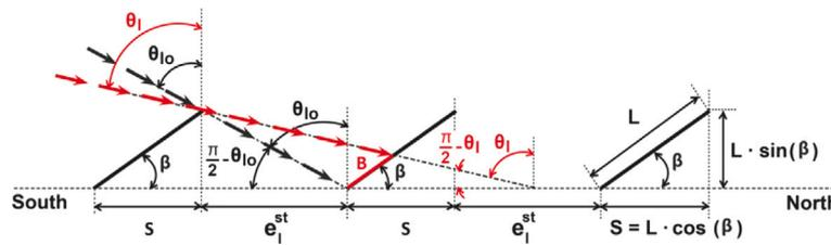
Fig. 5. Shading calculation.
