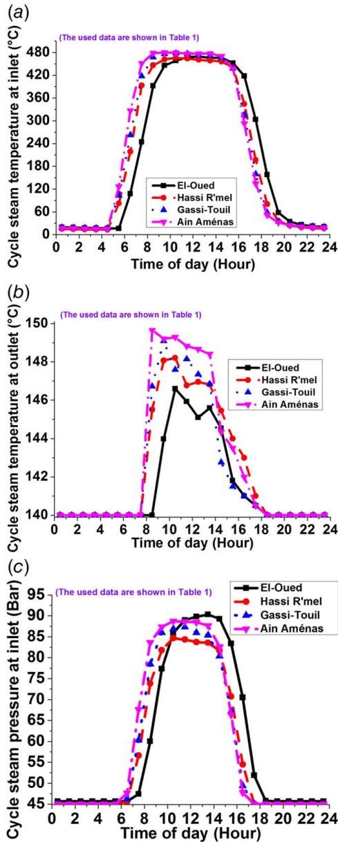
Fig. 5 Change in the operating parameters of the LFR power plants against time: (a) cycle steam temperature at RC inlet versus time, (b) cycle steam temperature at RC outlet versus time, and (c) cycle steam pressure at RC inlet versus time
