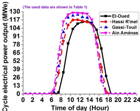
Fig. 6 Change in electrical power output against time
