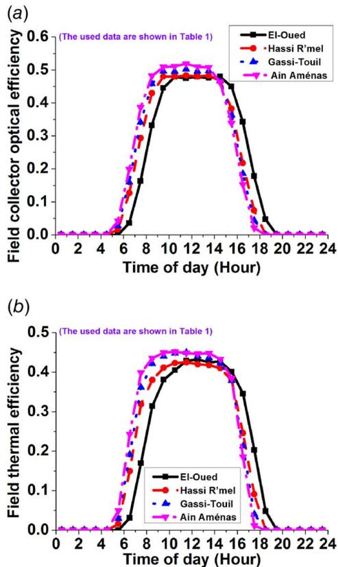
**Fig. 4** Field collector efficiency against time: (a) optical efficiency and (b) thermal efficiency
