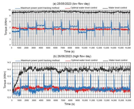
Figure 14. Time variation in the torque.
