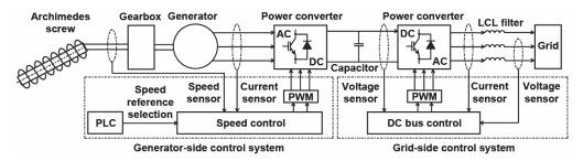
Figure 2. A micro-hydropower grid-connected control system.
