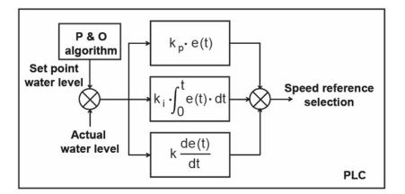
Figure 5. Diagram of an optimal water level control system.
