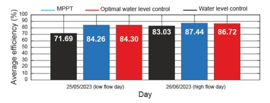
Figure 13. Average efficiency by the Barreda micro-hydropower plant using the three control systems.
