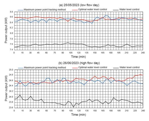
Figure 10. Power output by the Barreda micro-hydropower plant using the three control systems.
