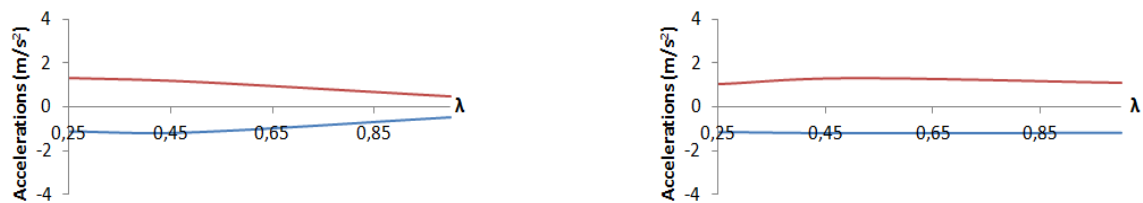
Figure 8: Maximum accelerations calculated at 1.8 meters far from the rail web. Circulation speeds of 30 km/h (left) and 70 km/h (right).
