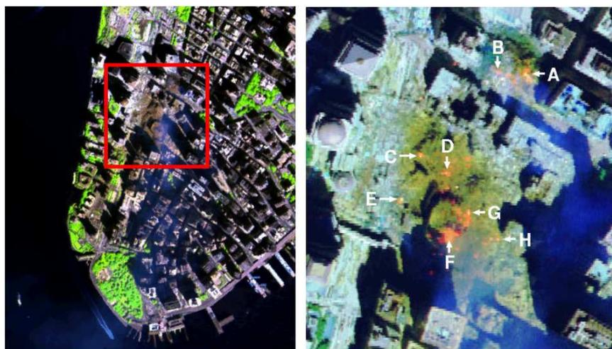
Figure 3: False color composition of an AVIRIS hyperspectral image collected by NASA's Jet Propulsion Laboratory over lower Manhattan on Sept. 16, 2001 (left). Location of thermal hot spots in the fires observed in World Trade Center area, available online: <http://pubs.usgs.gov/of/2001/ofr-01-0429/hotspot.key.tgif.gif> (right).
