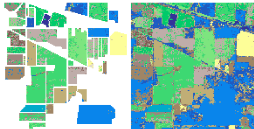
Figure 5: Classification results for the Small Indian Pines image: classification map without background (left) and classification map with background (right), obtained using 15% training.
