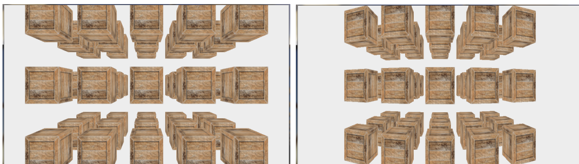
Figure 5: Scene rendered using symmetric view frustum with linear (left) and cylindrical (right) projections.
