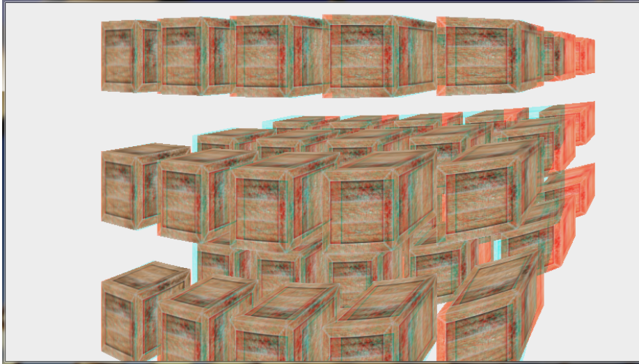
Figure 7: Stereoscopic rendering (red-cyan anaglyph) of the same scene using asymmetric view frustum with cylindrical projection.
