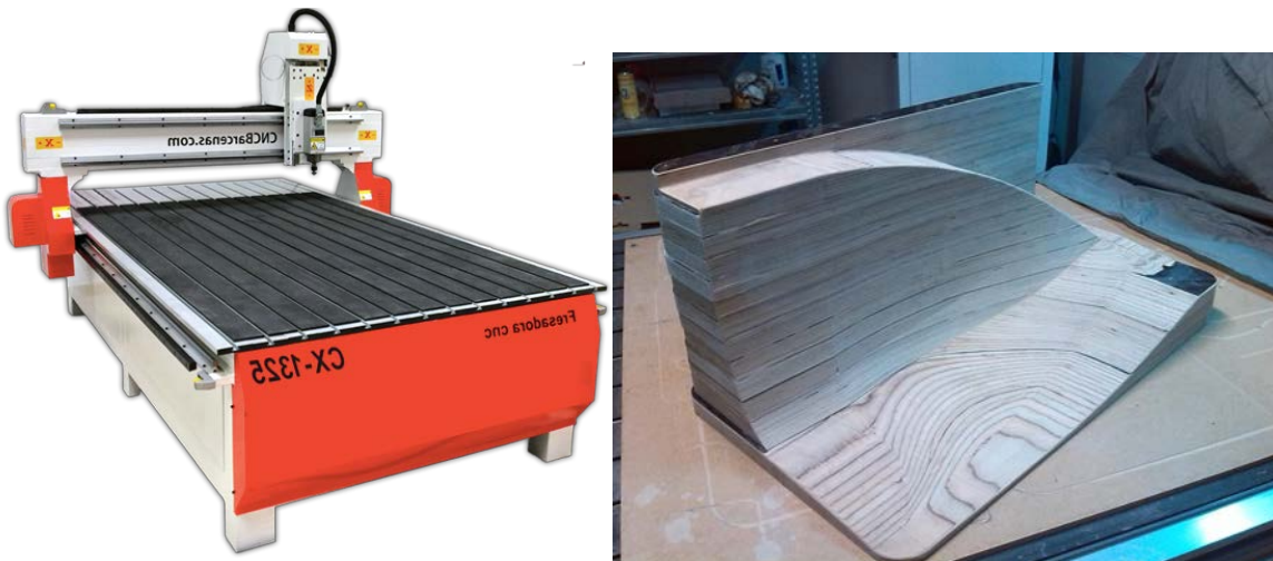
Figure. 9 Three-axis CNC equipment and pontoon part mold [5]
