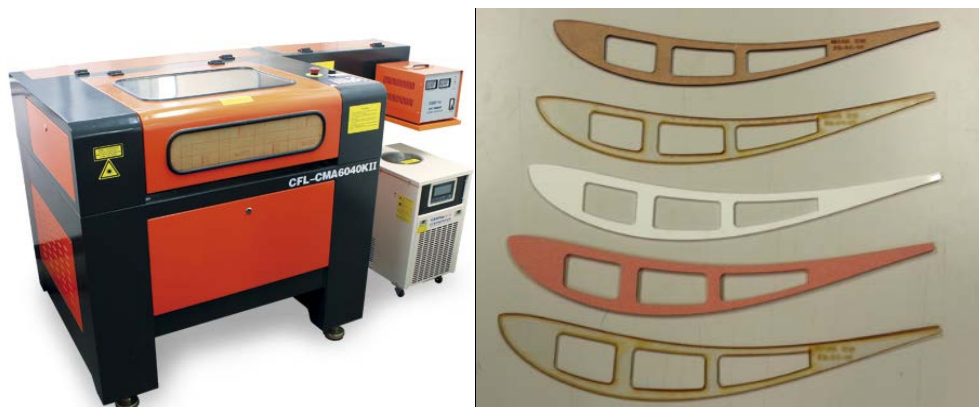
Figure 13. Laser CNC cutting machine (60 Wativos) and cut airfoil ribs
