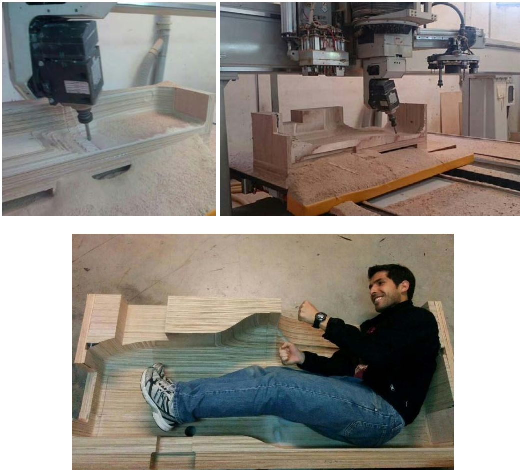
Figure 10. Monocoque manufacture with 5axes CNC machine (Hertalla [6])
