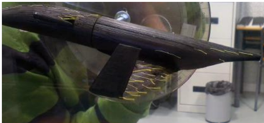
Fig. 1. Picture of the scale model built by the students and introduced in the wind tunnel. The mechanism to modify the angle of attack is depicted
