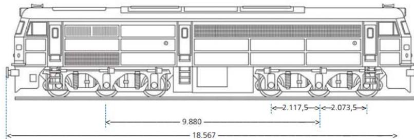
Fig. 2. Sketch and dimensions (mm) of the ALCO S321 locomotive used for this study
