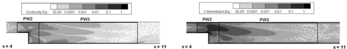
Figure 3: Contours of the local residuals (namely, the absolute value of the left hand side of the equation) of CFD solution at point PT3 in continuity (up) and x-momentum (down) equations
