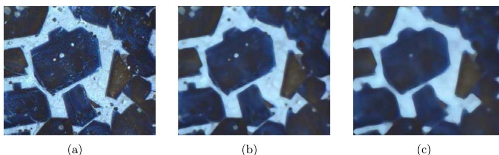
Figure 2: (a) the original clinker image. Note all the small elements that we do not really need to perform a segmentation. (b), the same filtered image using a median filter as proposed in text, with a neighbourhood distance  $N=4$ . (c), in this case, a neighbourhood distance of  $N=8$  is used. Note that as the neighbourhood distance is increased, more information is lost on small details.
