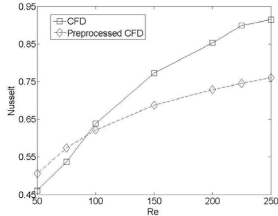
Figure 4: Nusselt number vs. Reynolds number resulting from CFD calculations, both with the code used in the remaining of the paper (solid) and with post-processing on the energy equation (dashed).
