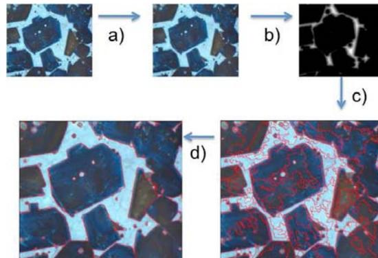
Figure 4: This image shows the proposed workflow for segmenting clinker images. It starts with a microscopic image of a clinker preparation. The filtering stage follows with the application of a median filter. Later, the gradient image is calculated as the input for the watershed algorithm. The last two images represent the oversegmented image and the fine-segmented result.
