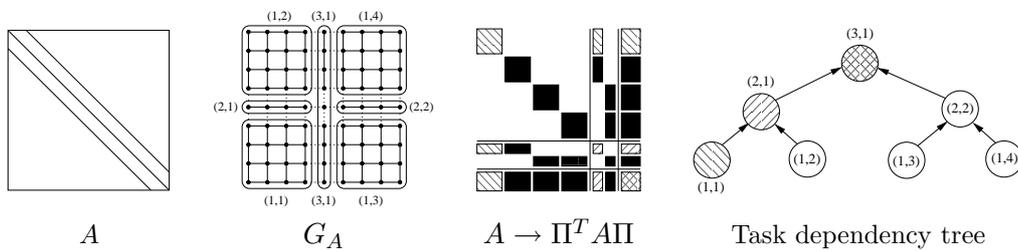
Figure 1: MLND partitioning. From left to right: natural ordering, nested dissection, nested dissection (re)ordering, and task dependency tree.
