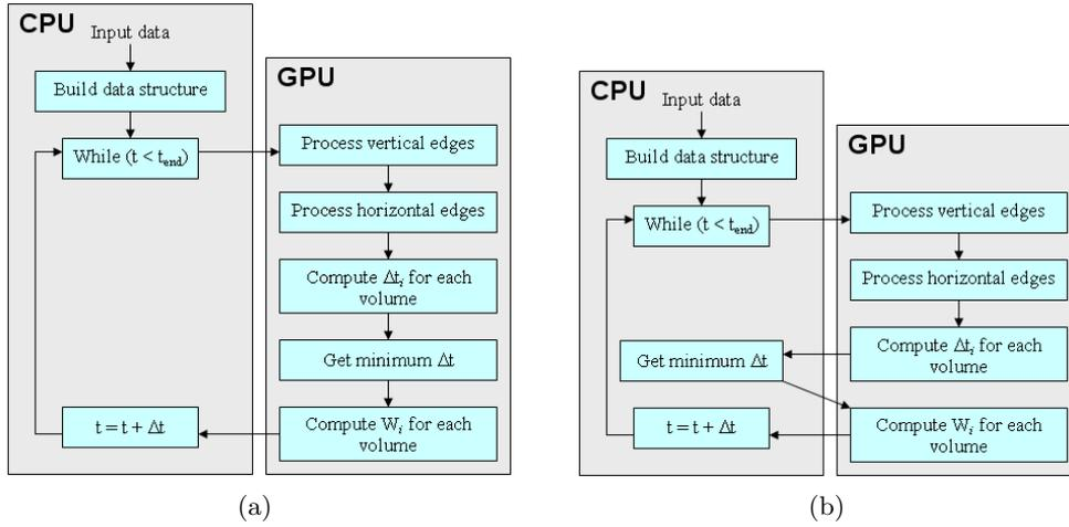
Figure 4: General steps of the parallel algorithm implemented in CUDA. (a) When there are more than a particular number of volumes, (b) Otherwise.
