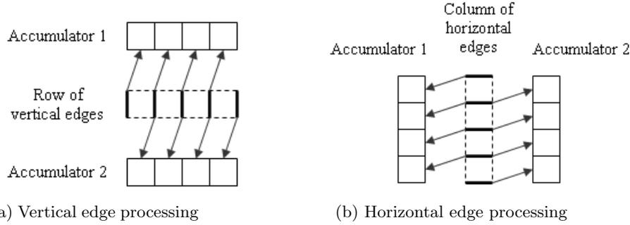
Figure 6: Computing the sum of the contributions of the edges of each volume.
