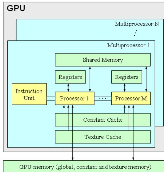
Figure 3: GPU architecture.
