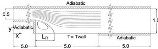
Figure 1: Sketch of the computational domain and the streamlines
