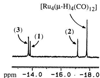
Fig. 2. Hydride region of the  $^1\text{H-NMR}$  spectrum of a sample obtained by thermolysis under nitrogen of a ca. 1:1 mixture of **2** and **3** in refluxing toluene for 2.5 h.
