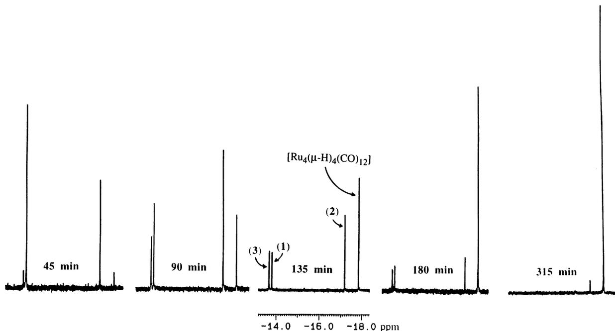
Fig. 1. Hydride region of the  $^1\text{H-NMR}$  spectra of samples obtained at different reaction times during the hydrogenation (1 atm) of compound **1** in refluxing toluene. The scale and peak assignments are only given in the central spectrum but are common to the five spectra.
