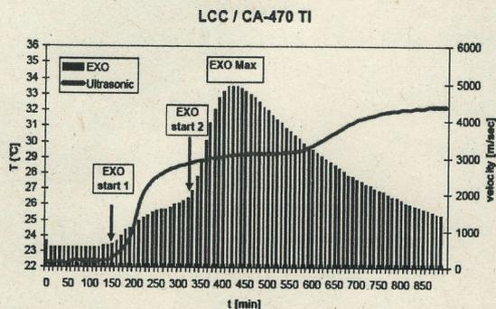
Figure 3. Measurement of setting by exothermic reaction and ultrasonic equipment.
