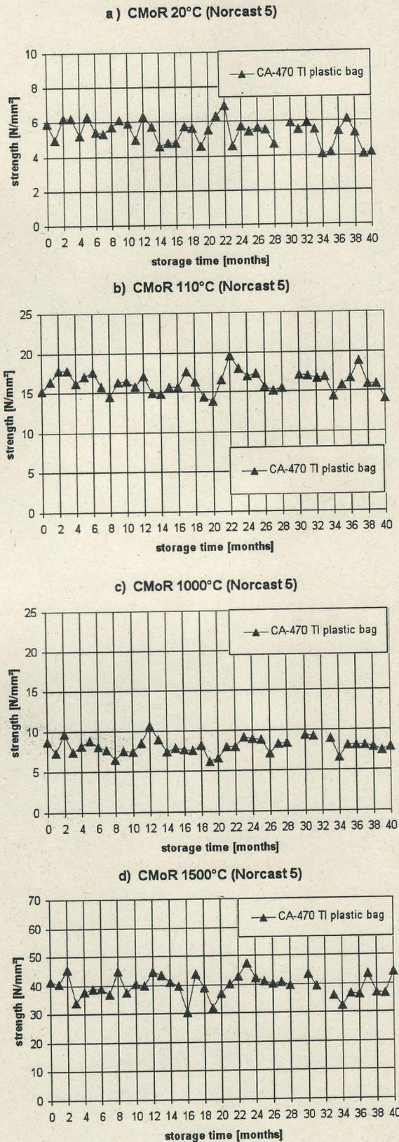
Figure 7 a-c. Impact of warehouse aging of plastic bagged CA-470 TI on strength of test castable (CMoR 20 – 1500 °C). See text regarding data point at 32 months.
