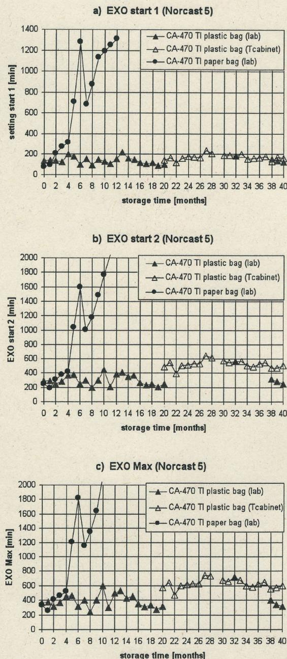
Figure 7 a-c. Impact of warehouse aging of CA-470 TI on setting (EXO start 1, start 2, and Max); plastic vs. paper bag. Measurement for CA-470 TI in plastic bags: phase 1 (0 – 21 months) in the lab and phase 2 (22 – 40 months) in a temperature cabinet at 20°C. See text regarding data point at 32 months.
