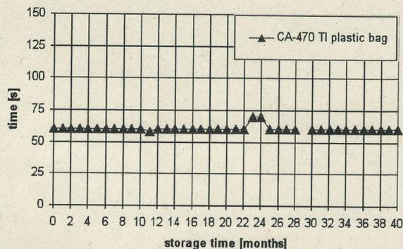
Figure 4. Impact of warehouse aging of plastic bagged CA-470 TI on wet out time. See text regarding data point at 32 months.
