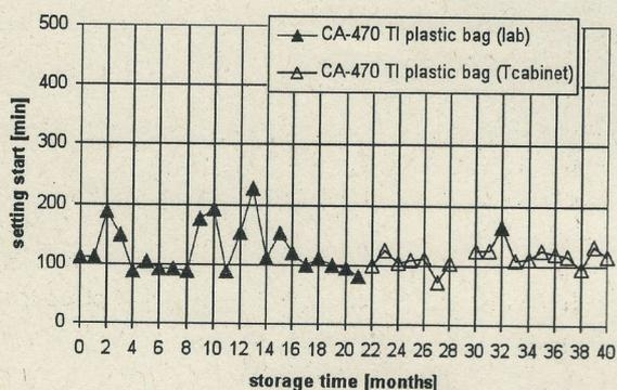
Figure 6. Impact of warehouse aging of plastic bagged CA-470 TI on ultrasonic setting start. Measurement phase 1 (0 – 21 months) in the lab and phase 2 (22 – 40 months) in a temperature cabinet at 20°C. See text regarding data point at 32 months.
