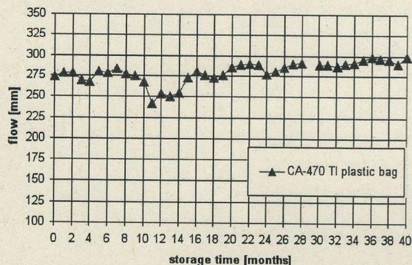
Figure 5. Impact of warehouse aging of plastic bagged CA-470 TI on flow at 10 and 30 minutes. See text regarding data point at 32 months.
