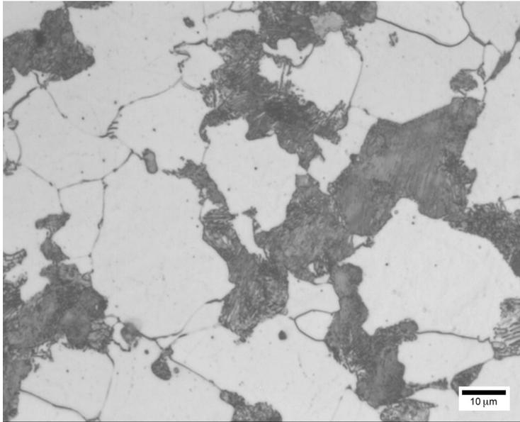
**FIGURE 5** Microstructure of the normalized (N) 8620 steel sample.
