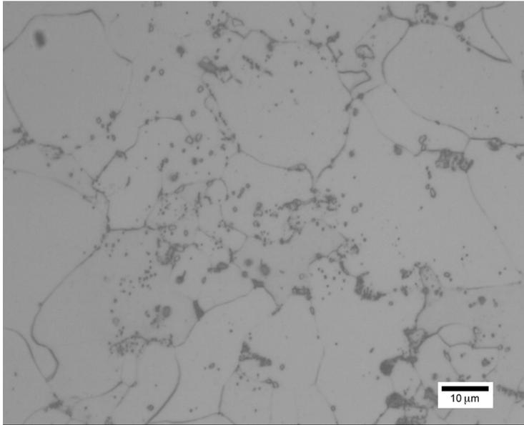
**FIGURE 2** Completely globulized pearlite microstructure (G).
