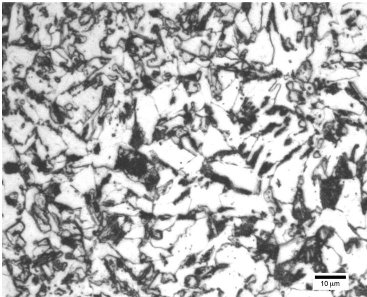
**FIGURE 3** Microstructure of the 8620 steel sample in the normalized and air-cooled (NA) state.
