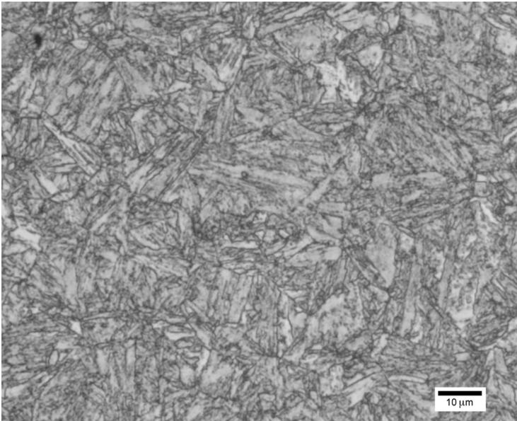
**FIGURE 8** Microstructure of the quenched and tempered (QT) sample.
