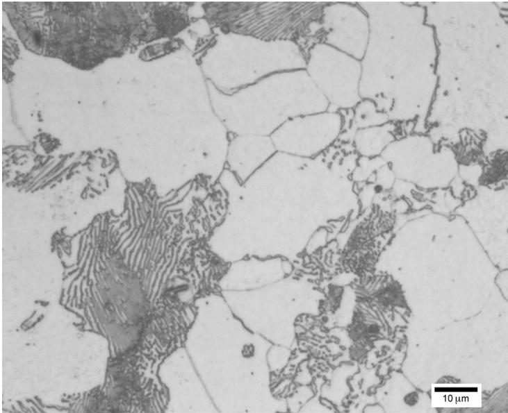
**FIGURE 7** Microstructure of the 8620 steel sample in the stress relieved (SR) state.
