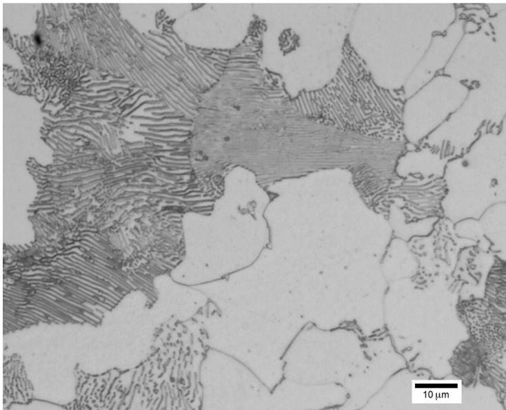
**FIGURE 6** Microstructure of the cold drawn (CD) sample initial state.
