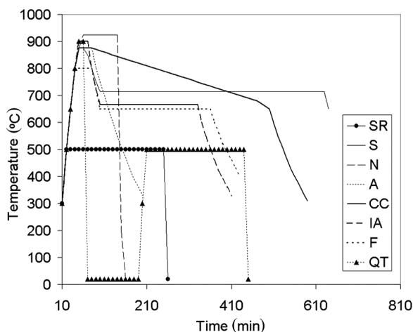
FIGURE 1 Heat treatments applied to 8620 steel samples.
