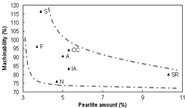
**FIGURE 9** Variation of machinability rate (MR) with amount of lamellar pearlite for different heat treated samples. The dotted lines indicate general behavior for this steel: a lower amount of pearlite is beneficial to machinability.
