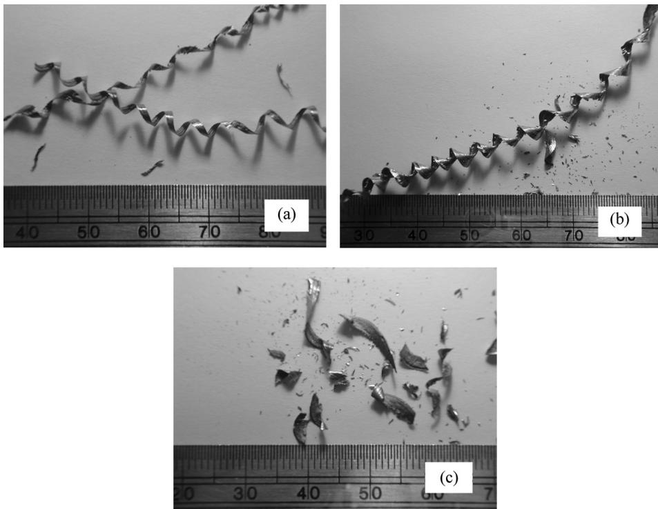
**FIGURE 10** Chip morphology for samples QT (a), S (b) and SR (c).
