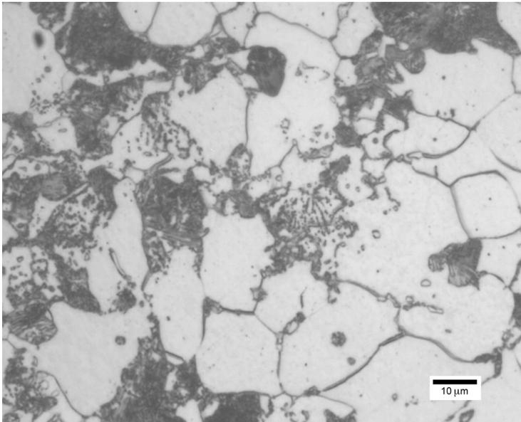
**FIGURE 4** Microstructure of the 8620 steel sample in the spheroidized (S) state.
