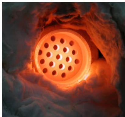
We propose in this publication the introduction of new, additional definition describing the multiple orifice ceramic filters used in research works on the liquid steel filtrations, calling this the filter slenderness ratio. Using this coefficient we obtain the possibility to compare the filtration effectiveness of different types of ceramic filters, not only for filters with cylindrical filtrating orifices, but also for other types, e.g., with orifices of rectangular section.
