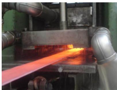
An experimental technique developed for monitoring the work roll surface temperature by sensors embedded in the work roll is presented. Continuous hot rolling pilot line trials were performed for different process conditions. These thermal measurements give very detailed information about the temperature field in the roll. The heat flux and heat transfer coefficient distribution along the roll circumference were obtained.
